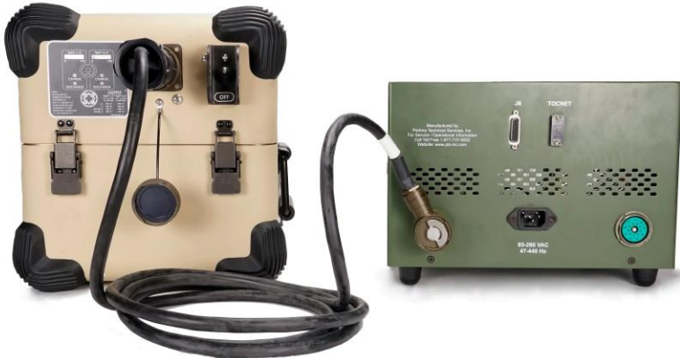
Power Supply connected to PSDS 24V DC Inputs. (Shown with CAB.DPW.101H connected)
