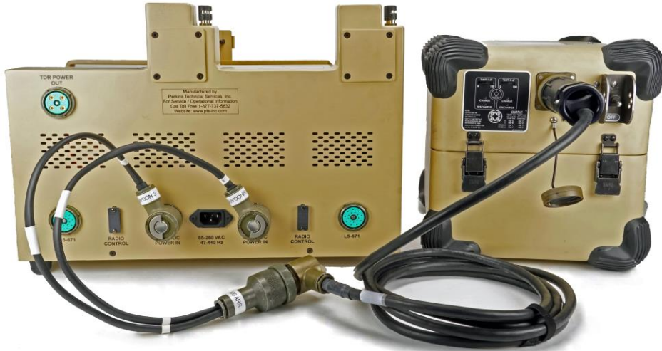
Power Source connected to PSDS 24V DC Inputs
