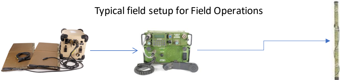
TOC Area Power Source & PSDS connected with 100' feedline (CAB.OTH.101)
