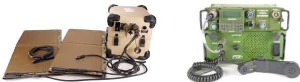
TOC Area Power Source & PSDS connected with 100' feedline (CAB.OTH.101)
