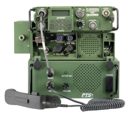
Attach the CAB.DPW.001(101.115.1500) Power cable to the back of the PSDS, 28V DC Power Out Connector and attach the RF-5833 to the DC Power Connector as shown on the photo.
