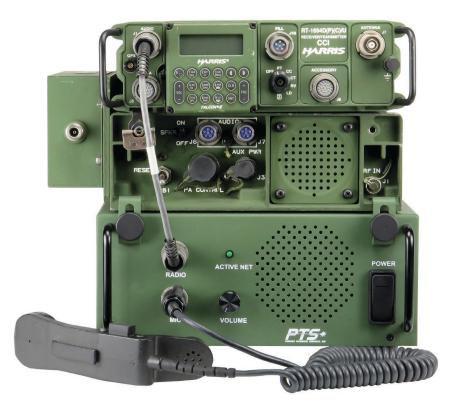
Attach the CAB.DPW.001(101.115.1500) Power cable to the back of the PSDS, 28V DC Power Out Connector and the RF-5833 to the DC Power Connector as shown on the photo.
