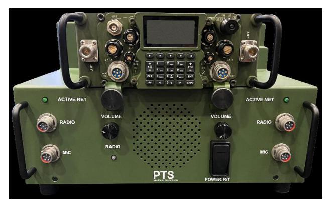
MODEL #: AS0162-CA-162 (Note: Radio in Picture Not Included) Includes 2 PTS-H-0003J Cable Compatible with 1 AN/PRC-162
