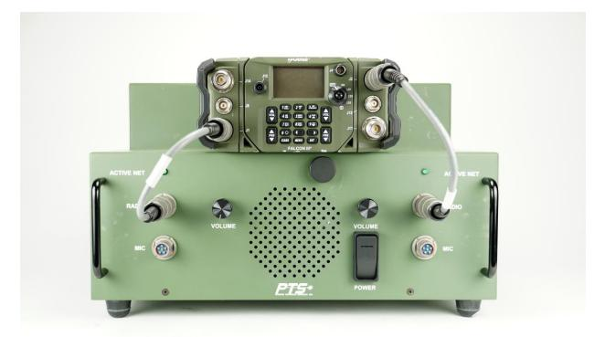
Turn the volume control counterclockwise to the stop. Adjust the volume knob to midrange. The radio handset volume affects speaker volume. The user will need to ensure the radio volume is adequate to drive the PSDS audio circuitry for proper operation. The user may now turn up the radio. The user will note that there is an ACTIVE NET LED for the NET. When transmitting or receiving the LED for the ACTIVE NET will illuminate green.
